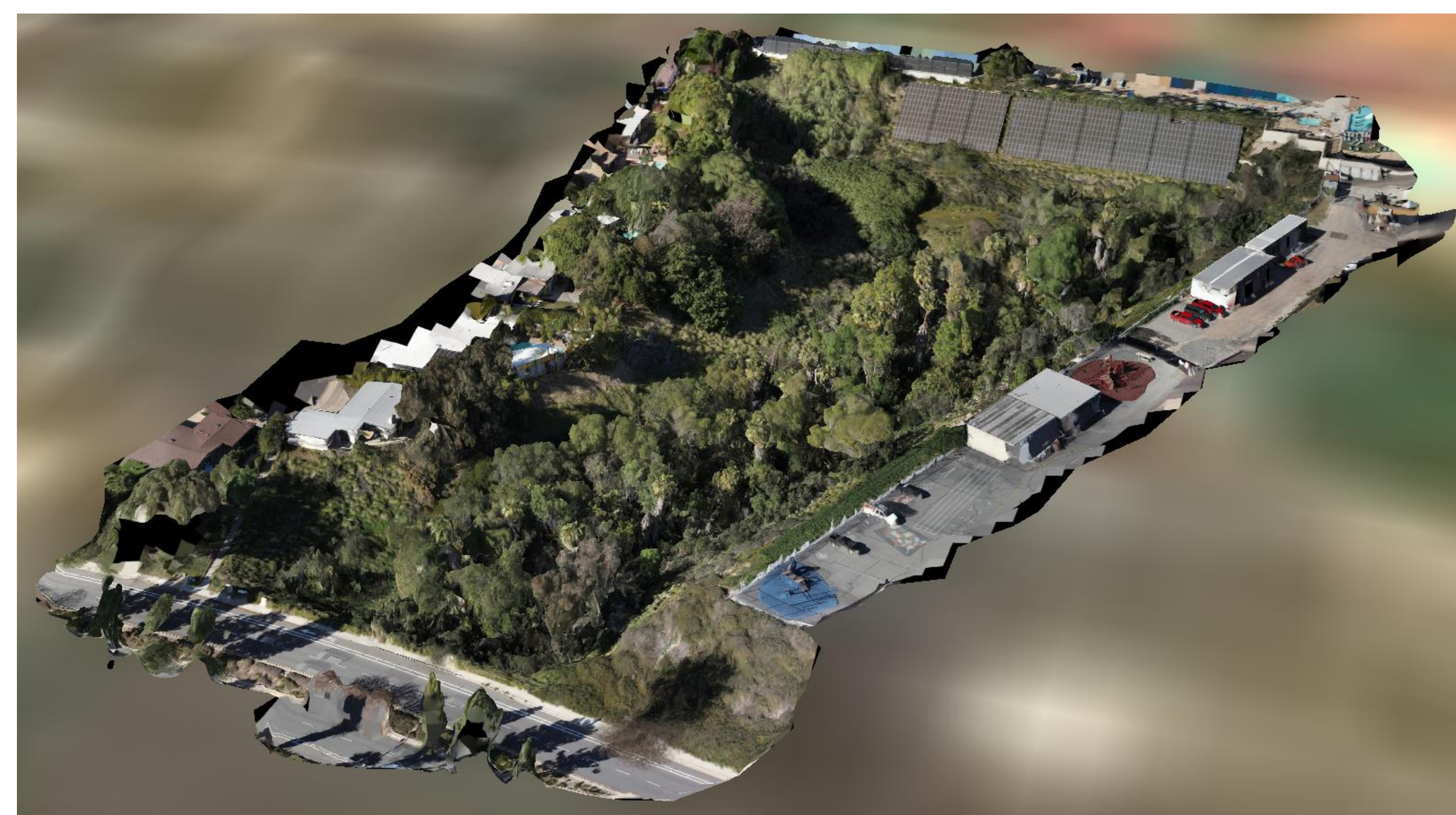
Image 5: SfM Photogrammetry of the canyon behind the Aquaplex. This was used to create the DEM model used to calculate valley erosional volume.
